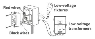
3. Connect field wires from transformer to dimmer wires (black). Connect fixture wires to dimmer wires (red).
