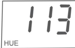
5. If GRP (Luxor Mode) is displayed, press the Mode **SEL** button to see the Hue, Saturation, or Intensity values.
