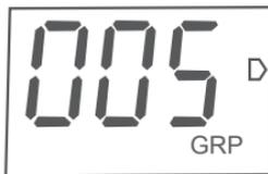
5. If HUE, SAT, or INT is displayed, press MODE
