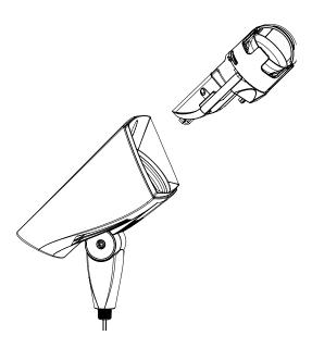
2. Lift the cartridge arm and turn it counterclockwise to release the lock. Pull the complete cartridge out of the fixture housing.
