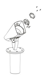
3. Unfasten the three LED module screws using a Phillips #1 screwdriver. Remove the reflector adapter ring and LED module.
