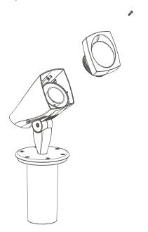
1. Remove the cap by unfastening the  $6-32 \times \frac{1}{2}$ " (13 mm) screw using a 764" Allen key. Then lift the cap outward. Avoid using metal tools while lifting the cap to protect the power coat finish.
