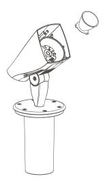
2. Twist the reflector optic counterclockwise and pull outward to remove.
