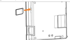
Figure 33: SD card installation
