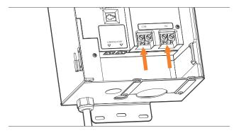
Figure 6: Output terminal blocks
