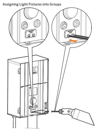
Figure 14: Fixture assignment wire diagram
