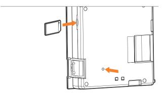
Figure 7: Back of facepack showing SD card and reset button
