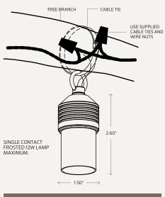
THIS FIXTURE IS DESIGNED FOR DOWN LIGHTING ONLY! DO NOT USE FOR UP LIGHTING.
